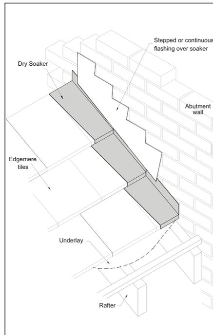
Fig 1 – Edgemere abutment with dry fix soakers
