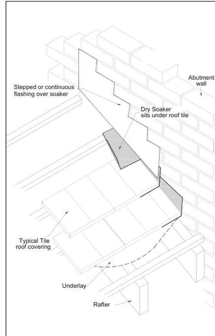
Fig 4 – Ashmore abutment with dry fix soakers
