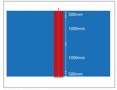
Fig. 6 - Fixing positions
