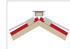
Fig. 9b - Ridge section below ridge tile
