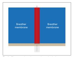
Fig. 2 – Place over breather membrane/underlay
