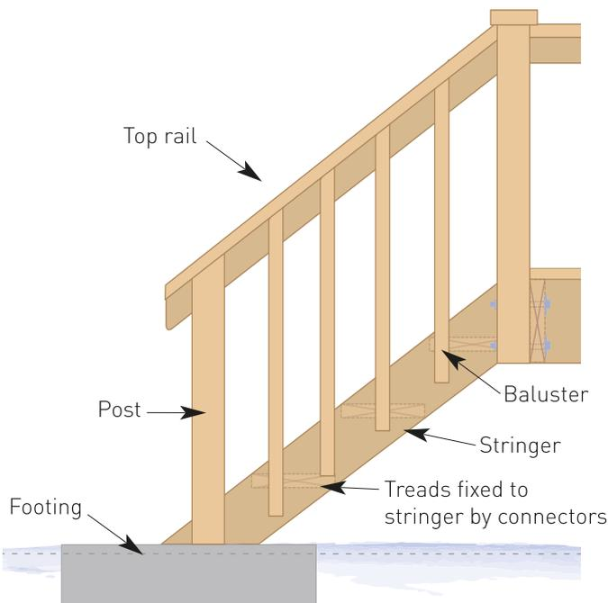
FIGURE 14: ATTACHMENT TO FOOTING
