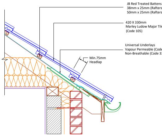
JB Red Treated Battens Machine Graded to BS5534 38mm x 25mm (Rafters 400mm - 450mm) 50mm x 25mm (Rafters 450mm - 600mm)
