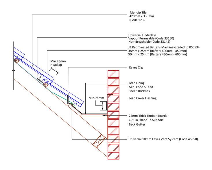
Ventilated Lead Back Gutter
