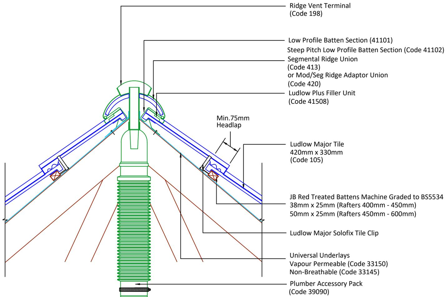
\*Cover Batten Section slots with Blanking Tape (Code 33001) for a distance of at least 600mm either side of the vent.
