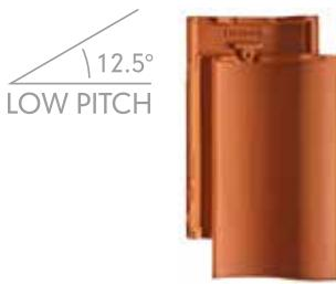
Melodie is a single interlocking clay pantile with a flexible gauge and a robust interlock, enabling it to perform at pitches as low as 12.5°. Available in a Natural Red colour.
