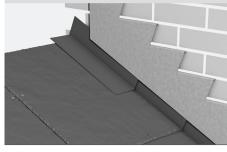
The Marley range of individual dry soakers is an easy to install, lightweight and highly affordable way to reduce both the material and labour costs associated with lead at side abutments.
