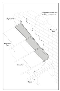
Fig 1 – Edgemere abutment with dry fix soakers
