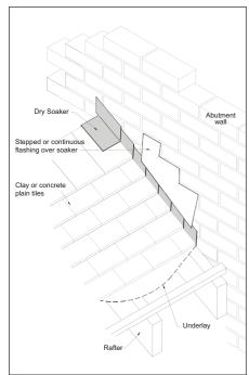
Fig 3 – Clay or concrete plain tile abutment with dry fix soakers
