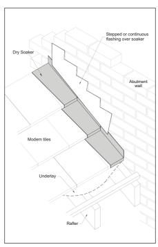
Fig 2 - Modern abutment with dry fix soakers
