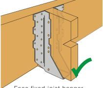
Face fixed joist hanger. Always fasten with nails or screws made from the same material
