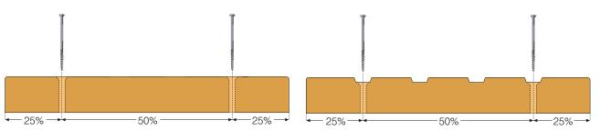
Fixing points on boards should be positioned 25% in from each side. On grooved boards the fixing point is at the bottom of the groove.
