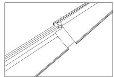
Fig. 9 - Slide verge units upwards
