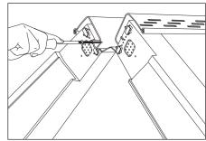
Fig. 11 - Screw verge units at apex of verge
