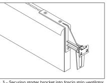
Fig. 3 - Securing starter bracket into fascia strip ventilator
