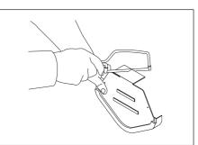
Fig. 17 – Cutting end cap flange
