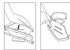
Figs. 12 and 13 – Cutting end cap flange
