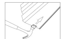
Fig. 7 – Securing the first verge with mechanical fixing
