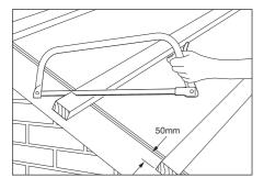
Fig. 1 – Position top course tiling battens
