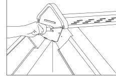
Fig. 14 – Screw fix ridge end cap
