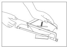
Fig. 16 – Cutting end cap flange
