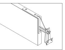
Fig. 2 – Securing starter bracket onto corner of fascia
