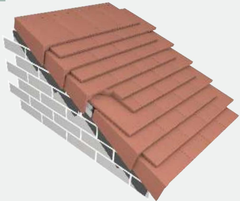
Plain tile cloak verges provide a weatherproof and mortar free finish to the roof verge. They are available in right and left hand units in colours to match the main roof tiles, twice nailed for maximum security. The apex of the roof is finished with matching stop-end ridge tiles.
