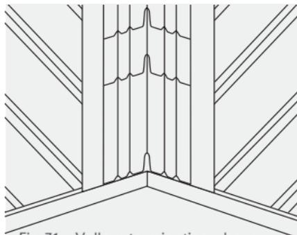
Fig 71 – Valleys terminating above eaves level
