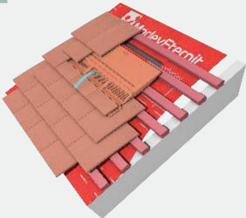
Available in a range of bases with real clay tile slips on the visible edge (3 tiles wide). The clay tile vent provides a net ventilation area of 7,500mm<sup>2</sup> per vent. Suitable for natural, mechanical or soil pipe ventilation.
