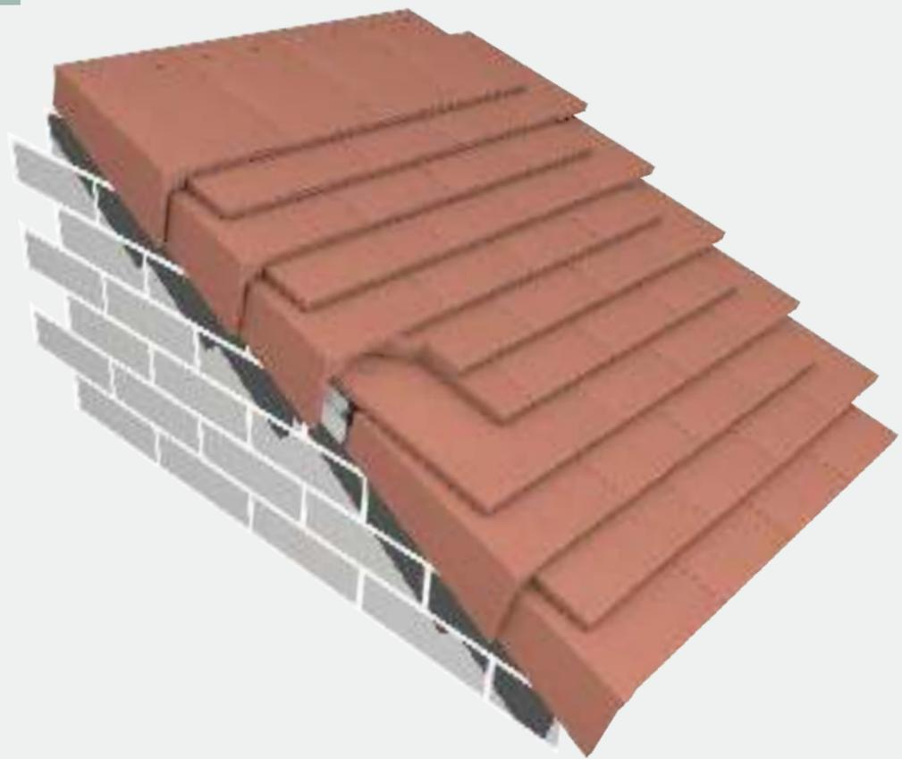
Plain tile cloak verges provide a weatherproof and mortar free finish to the roof verge. They are available in right and left hand units in colours to match the main roof tiles, twice nailed for maximum security. The apex of the roof is finished with matching stop-end ridge tiles.
