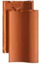
Melodie is a single interlocking clay pantile with a flexible gauge and a robust interlock, enabling it to perform at pitches as low as 12.5°. Available in a Natural Red colour.
