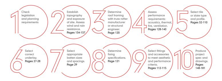
Reference should also be made to the latest versions of BS 5534 'Slating and tiling for pitched roofs and vertical cladding – Code of practice)', and to BS 8000: Part 6: 'Workmanship on Building Sites: Code of Practice for slating and tiling of roofs and claddings' and BS 5250 'Code of practice for control of condensation in buildings'.
