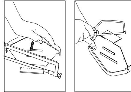
Figs. 9 and 10 – Cutting end cap flange
