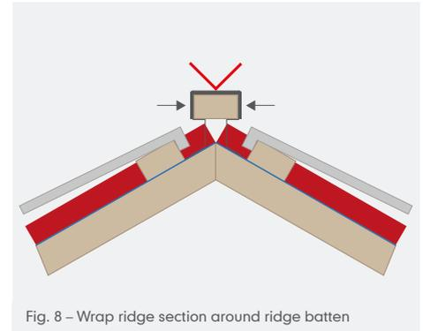
Fig. 8 – Wrap ridge section around ridge batten
