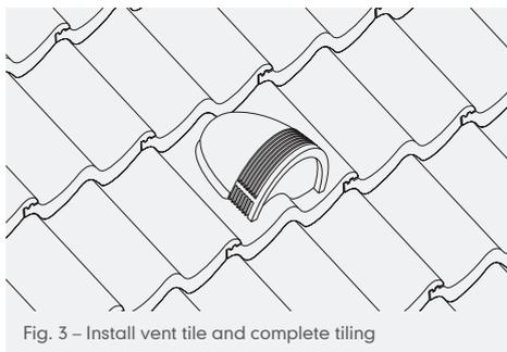
Fig. 3 - Install vent tile and complete tiling
