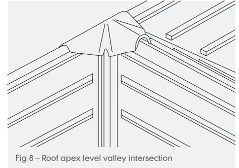
Fig 8 – Roof apex level valley intersection
