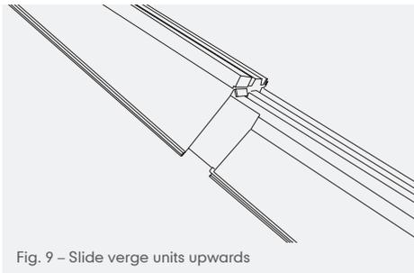
Fig. 9 – Slide verge units upwards
