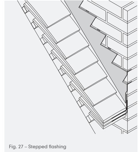
Fig. 27 – Stepped flashing
