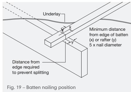
Fig. 19 – Batten nailing position
