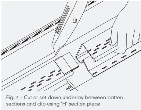
Fig. 4 – Cut or set down underlay between batten sections and clip using 'H' section piece
