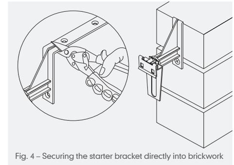
Fig. 4 – Securing the starter bracket directly into brickwork
