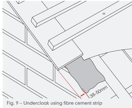
Fig. 9 – Undercloak using fibre cement strip
