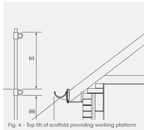
Fig. 4 – Top lift of scaffold providing working platform
