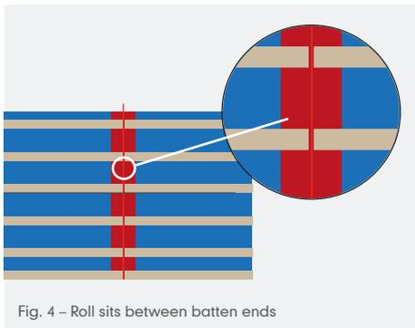
Fig. 4 – Roll sits between batten ends
