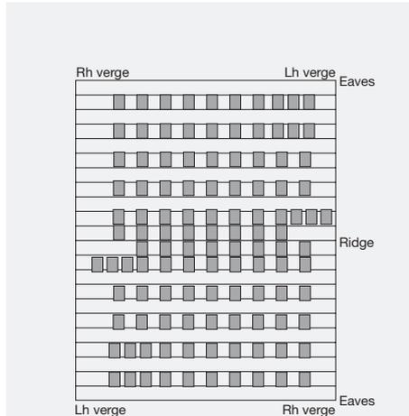
Fig. 6 – Loading roof evenly with tile/slate stacks
