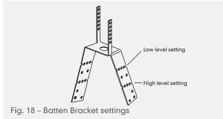
Fig. 18 – Batten Bracket settings
