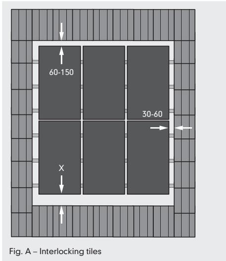
A Interlocking tiles – set lower gap ‘X’ 130-150mm above the head of the tile.
