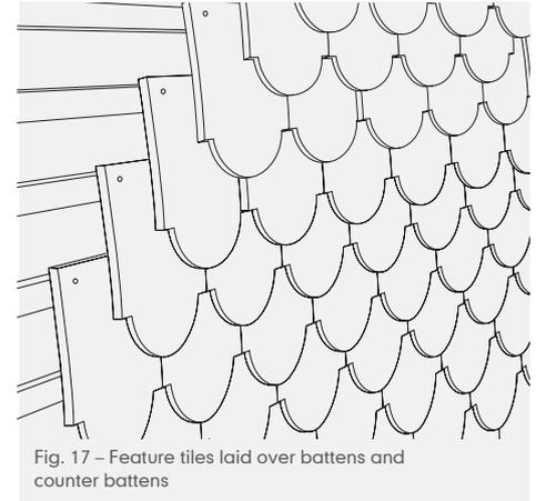
Fig. 17 – Feature tiles laid over battens and counter battens
