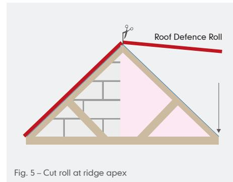
Fig. 5 – Cut roll at ridge apex
