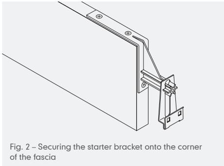
Fig. 2 – Securing the starter bracket onto the corner of the fascia
