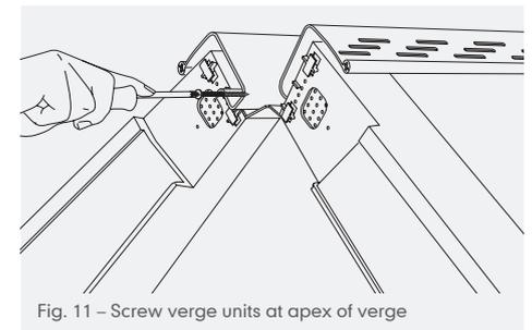
Fig. 11 – Screw verge units at apex of verge
