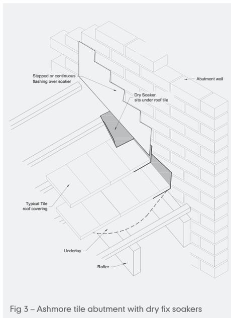
Fig 3 – Ashmore tile abutment with dry fix soakers
