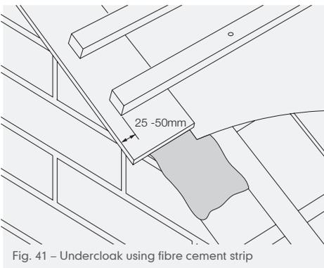
Fig. 41 – Undercloak using fibre cement strip
