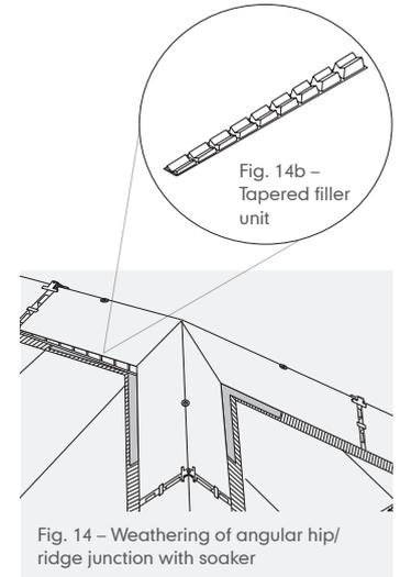
Fig. 14b – Tapered filler unit
