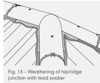
Fig. 13 – Weathering of hip/ridge junction with lead soaker
