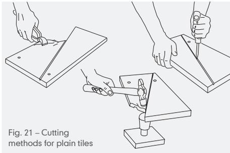
Fig. 21 – Cutting methods for plain tiles
