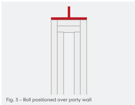
Fig. 3 – Roll positioned over party wall
