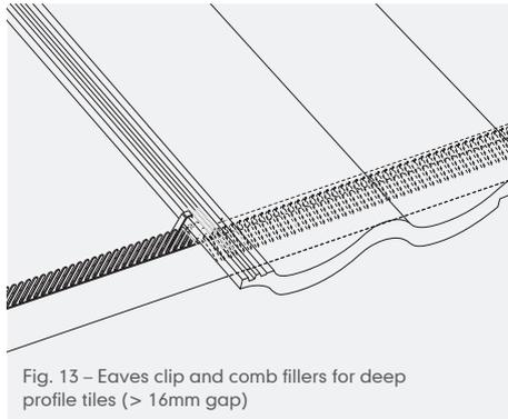
Fig. 13 – Eaves clip and comb fillers for deep profile tiles (> 16mm gap)
