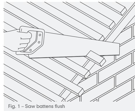
Fig. 1 – Saw battens flush
