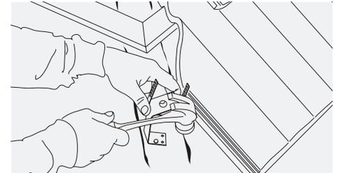
Fig. 2 – Fixing hip batten brackets
