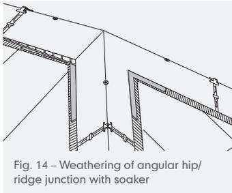
Fig. 14 – Weathering of angular hip/ridge junction with soaker
