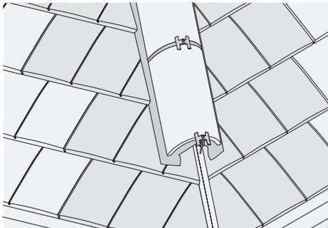
Fig. 20 – Typical bedded hip using third round ridge units as hip capping, tile-and-a-half tiles shown shaded
