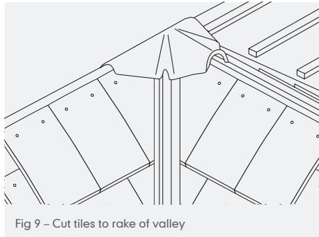
Fig 9 – Cut tiles to rake of valley
