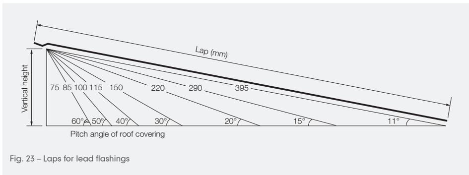
Fig. 23 – Laps for lead flashings
