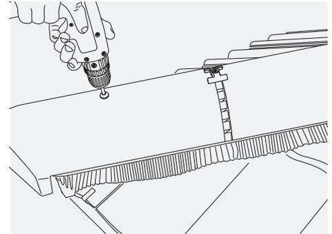
Fig. 31 – Mechanically fixed hip end using HipFast system
