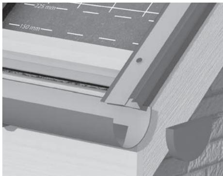
Fig. 19 – Nail each length of trim to batten
