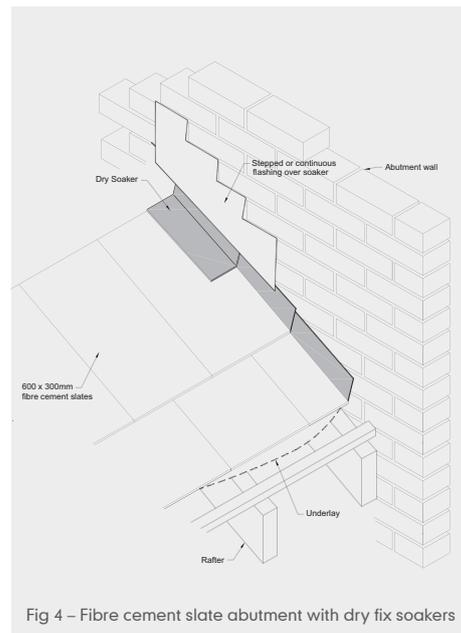
Fig 4 – Fibre cement slate abutment with dry fix soakers
