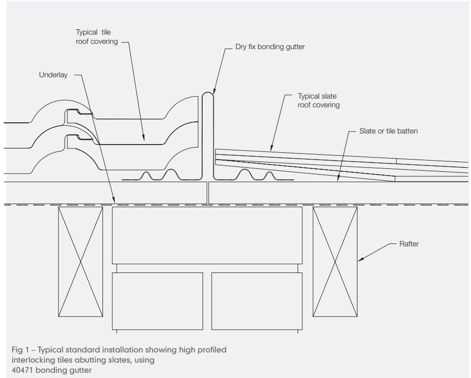
Fig 1 – Typical standard installation showing high profiled interlocking tiles abutting slates, using 40471 bonding gutter
