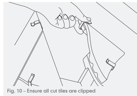
Fig. 10 – Ensure all cut tiles are clipped
