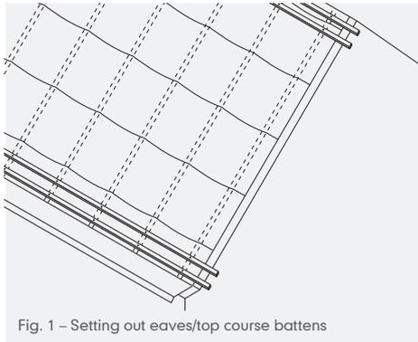
Fig. 1 – Setting out eaves/top course battens
