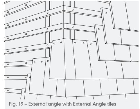
Fig. 19 – External angle with External Angle tiles
