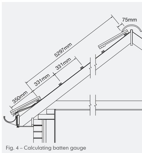
Fig. 4 – Calculating batten gauge
