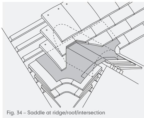
Fig. 34 – Saddle at ridge/roof/intersection
