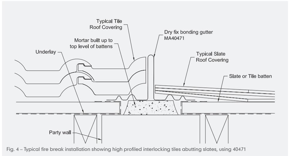
Fig. 4 – Typical fire break installation showing high profiled interlocking tiles abutting slates, using 40471
