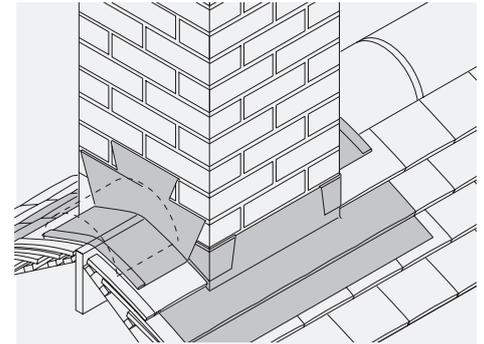
Fig. 32 – Roof chimney at ridge line
