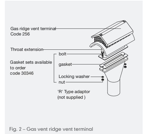
Fig. 2 – Gas vent ridge vent terminal
