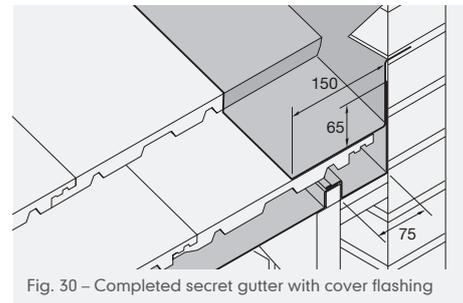
Fig. 30 – Completed secret gutter with cover flashing
