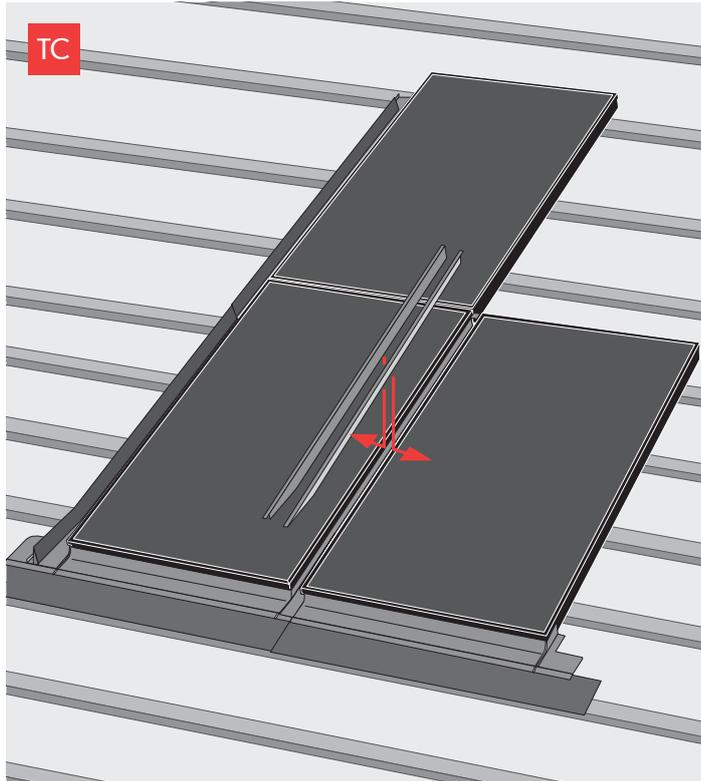
TIP: Installing the combi-batten brackets and the upper gutter before the lower gutter covers, can make this part of the installation quicker and more straightforward.
