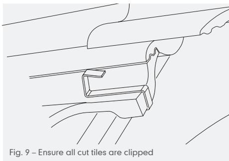
Fig. 9 – Ensure all cut tiles are clipped
