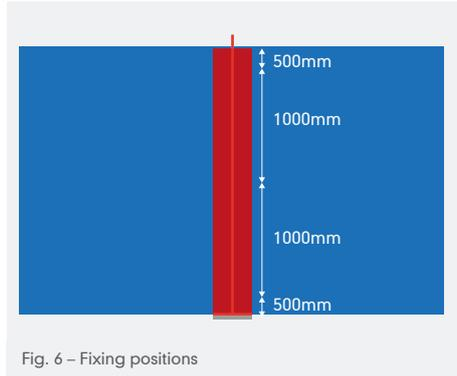
Fig. 6 – Fixing positions
