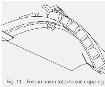
Fig. 11 – Fold in union tabs to suit capping
