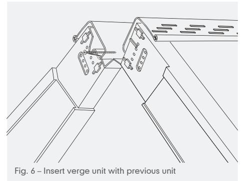
Fig. 6 – Insert verge unit with previous unit
