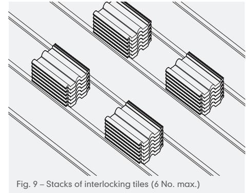
Fig. 9 – Stacks of interlocking tiles (6 No. max.)
