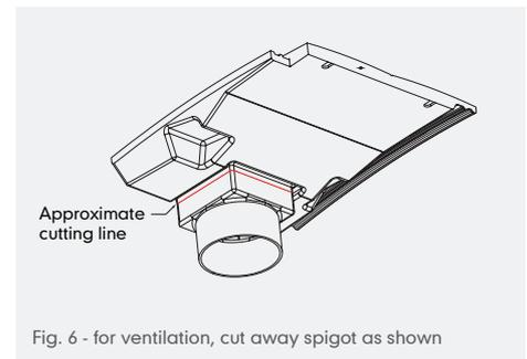
Fig. 6 - for ventilation, cut away spigot as shown
