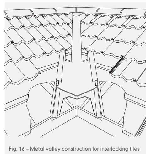
Fig. 16 – Metal valley construction for interlocking tiles
