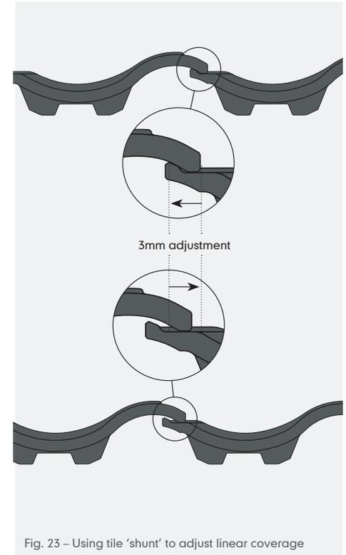
Fig. 23 – Using tile 'shunt' to adjust linear coverage
