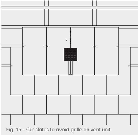
Fig. 15 – Cut slates to avoid grille on vent unit
