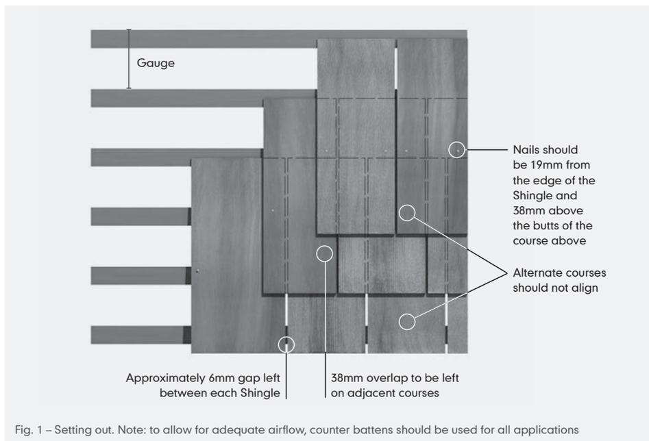
Fig. 1 – Setting out. Note: to allow for adequate airflow, counter battens should be used for all applications
