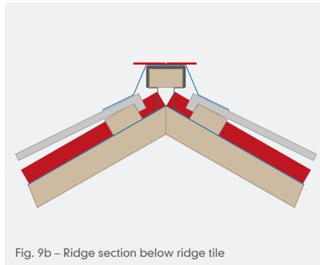
Lift one side of the breather membrane and fold the two halves of the upper roll pad together and gently insert these two halves of the pad through the incision and then fold the ridge section down over the ridge kit breather membrane.
