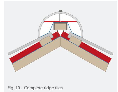
The upper strip of roll should now be sitting over the breather kit membrane in a position that will be beneath the ridge tile.
