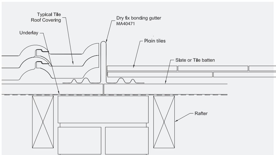
Fig. 3 – Typical standard installation showing high profiled interlocking tiles abutting slates, using 40471
