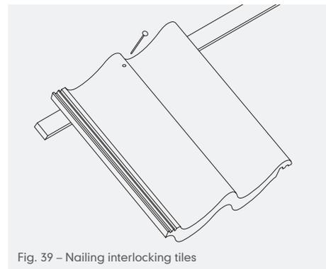
Fig. 39 – Nailing interlocking tiles
