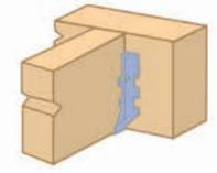
Joists can be face fixed to wall plates and beams using a suitable joist hanger
