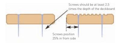
Screw heads should be countersunk level with the surface of the board or just slightly below the surface if the board has a moisture content higher than the equilibrium moisture content at the site – see section 1.6.
