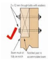
Soild beam Beam must sit fully on notch.
