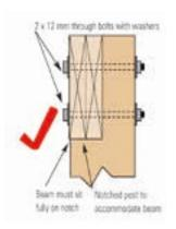
Double beam Notched post to accommodate beam
