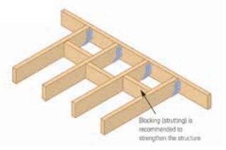
Joists adjacent to other load-bearing components such as beams and newel post fixing point should always be blocked – see Figure 11 on page 15.
